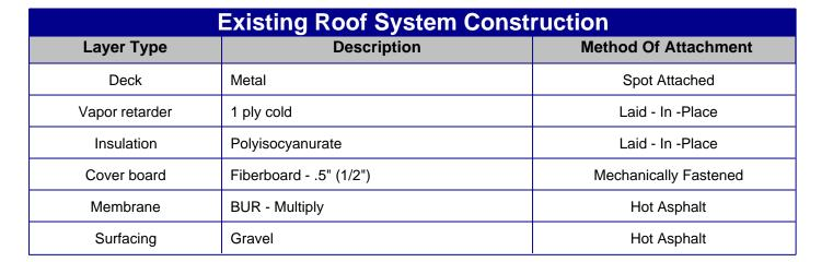
One (1) core cut revealed a steel decking and a single ply vapor barrier. The insulation consists of one (1) layer of 1" polyisocyanurate board and one (1) layer of .5" wood fiber cover board. The membrane is a multiply BUR with a gravel surface.
