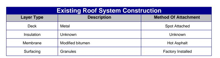
Due to the relatively recent application of the roof system, no core sample was taken on this roof section. An under view of the structure revealed a factory primed steel decking. The membrane is a SBS modified bitumen with a granulated surfacing.
